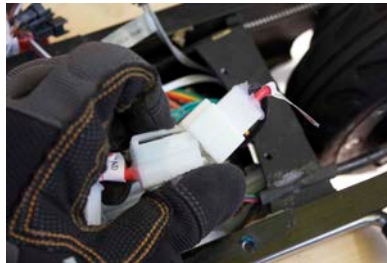
A3. Cut off all the cable tights on the connectors. Disconnect the connectors with the following labels: 1.Load and 6.Charge.
