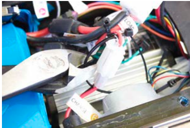
A3. Cut off all the cable tights on the connectors. Disconnect the connectors with the following labels: 1.Load and 6.Charge.
